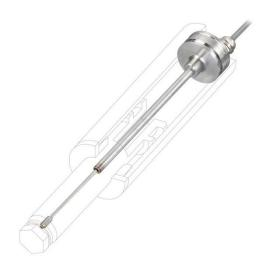
Furthermore, with a transducer body of only 8mm the ICT800 & 820 are well suited for use on small-bore actuators; while offering a choice of internal or threaded external flange mounting configurations to suit tie-rod, welded and rear clevis-mounted cylinder types in stroke ranges from 25 to 1000mm.
